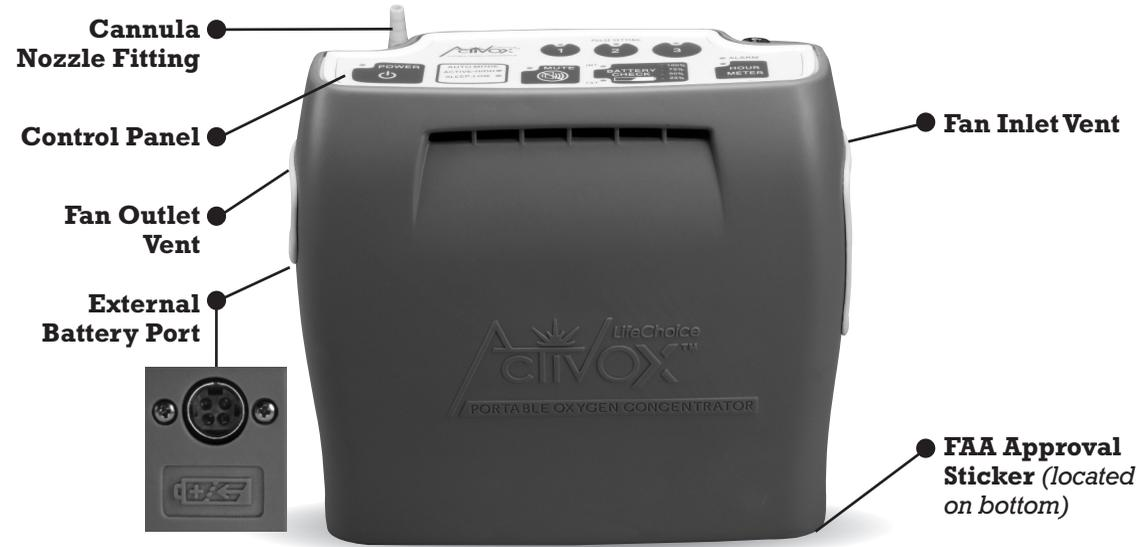
**Cannula Nozzle Fitting:** The nasal cannula connects to the oxygen output nozzle at the top of the LifeChoice Activox POC. Do not place the cannula into nasal passages until the LifeChoice Activox POC is fully powered on. Breathing through the cannula during start-up will prevent the system from powering on.
