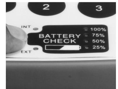
When the LifeChoice Activox POC is being powered from the internal battery, the Battery Check LED labeled INT will be slowly flashing. Pushing the Battery Check Button will display the charge level of the internal battery.
