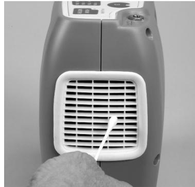
At least once a month inspect the grille of the intake vent and if it appears dirty, use a dry cotton swab (Q-Tip® or similar) to clean it. Never use alcohol, solvents, or petroleum distillates for cleaning.
