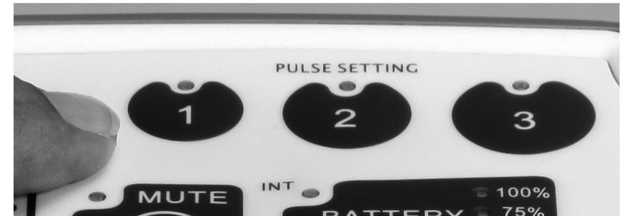
6. Place the nasal cannula in the nasal passages and breathe normally. When the LifeChoice Activox POC senses inhalation, oxygen is supplied through the cannula. The duration and size of the pulse is dependent upon the Pulse Setting selected.
